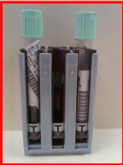
Twisted labels, and labels placed too low on the tube cannot be read by the instrument
