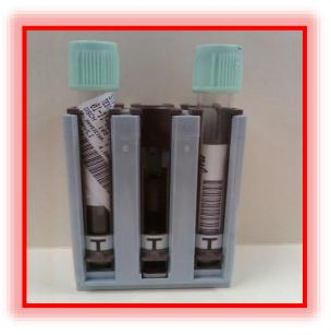
Twisted labels, and labels placed too low on the tube cannot be read by the instrument
