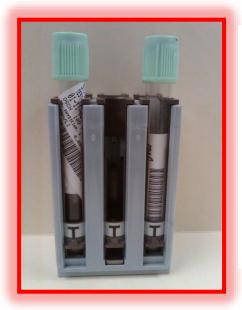
Twisted labels, and labels placed too low on the tube cannot be read by the instrument
